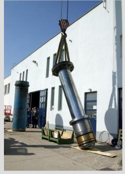
Field of use: Hydraulic cylinder for waste compression
