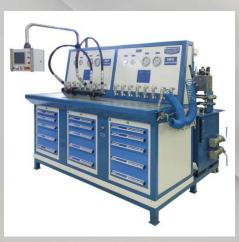
In-house built hydraulic cylinder test machine with data collection system. Cylinders can be certified on demand.
